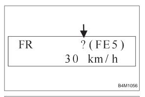
2) If freeze frame data is not properly stored in memory (due to a drop in ABSCM power supply, etc.), a trouble code, preceded by a question mark "?", appears on the select monitor display. This shows it may be an unreliable reading.
