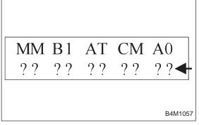
3) When a trouble code is detected in the FE mode, a question mark "?" appears continuously on the select monitor display until the freeze frame data is stored in memory.
